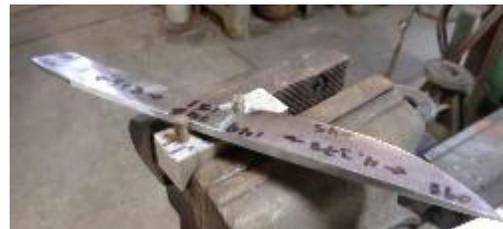
a scribed line. Use a center punch to mark the locations of the holes. If there are two scribed lines, just split the difference when making the punch marks.
