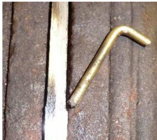
The tang is then ground – either in a taper spine-to-bottom or a quasi-rectangle. You want the sides to be flat and symmetrical side-to-side.
