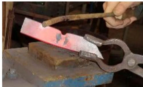
We can now do a preliminary shaping on the tang. The tang is placed on the anvil with the tong hand down enough to "catch" the depression on the edge of the anvil. Strike at the spine of the tang to "spread" the depression out. Do not worry about the fact that the narrowing of the tang as it meets the blade is far too fat. This is a good thing. The blade end won't flop around excessively when
