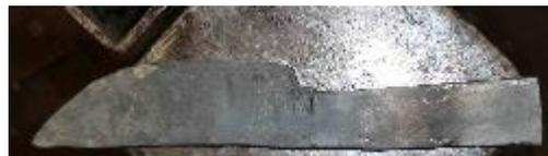
Here the tang before significant forging is compared to the model. The tang is shorter than the model's tang.
