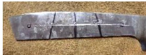
Drill the holes on the drill press. The holes need to be a touch bigger than the pin stock, so here they are made with a #30 drill bit (0.128") for use with 1/8" stock. Remember to compensate for the tapers spine-to-bottom, front-to-back when locking the tang in the drill press vise. The image here shows the balance point is about right, the holes are done, and the tang surface needs a touch more grinding (the little extension of the cliff wall forward onto the blade surface).
