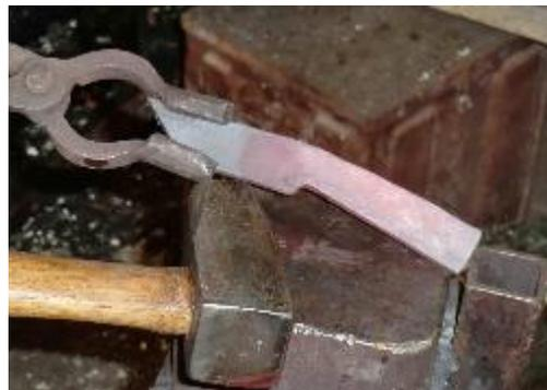
First, beat in the angle formed by the diagonal cut and the edge (Ok, we missed that picture, so live with it). The metal will thicken at the angle, so flip it on the side and push it back to the original thickness. Repeat until you like the curve from the main part of the edge to the tip. You now have a profile established.
