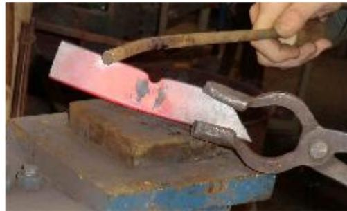
We can now do a preliminary shaping on the tang. The tang is placed on the anvil with the tong hand down enough to "catch" the depression on the edge of the anvil. Strike at the spine of the tong to "spread" the depression out. Do not worry about the fact that the narrowing of the tang as it meets the blade is far too fat. This is a good thing. The blade end won't flop around excessively when
