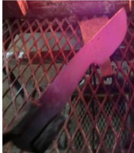
The last step is to anneal the blade. Run it back up to critical and then bury it in either wood ash (here in an old ammo container) or
