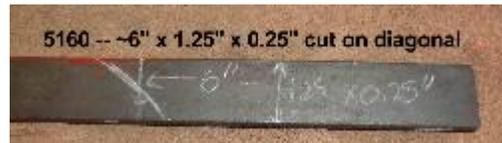
Why forge the corner back into the body to make the tip when a diagonal cut does most of the work? As shown, the blank has 1.85 in<sup>3</sup> of volume and the projected blade needs only 1.5 in<sup>3</sup>, so there is ample “meat” for our purposes.
