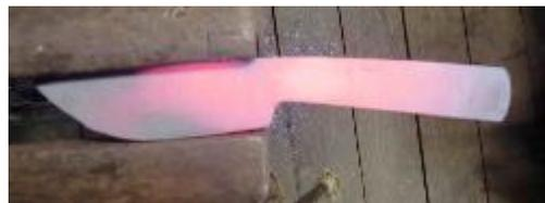
The more dings in the tang, the more work in the fit-&-finish. If you have a treadle hammer and a flatter, use them. It pays off in the long run. Remember that if you do the drop handle and/or use a flatter, make sure the blade and tang are still in line and that the tapers are symmetrical to their center lines.
