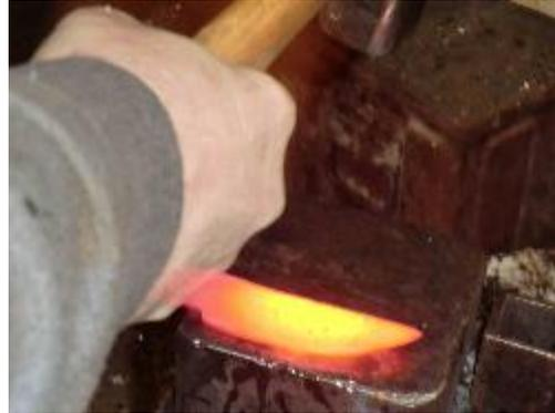
When the rough forging is completed on the blade, there ought to be an obvious taper from tip to tang as shown.
