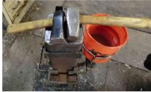
The first critical decision is the steel type. What is being used here is 5160, a nice friendly steel but any high-carbon forgeable steel is ok (L6, O1, 1095, 52100, etc.). You will want a bar slightly larger than the desired final dimensions. In this case, it's 1.25" x 0.25" while aiming for a 1" x 3/16" blade. Note the diagonal mark.
