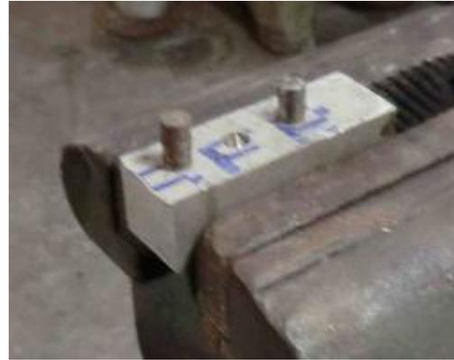
Lay the blade between the flanking pins and draw the blade between them while maintaining downward pressure. In this image, the spine is being pressed to the left pin, it is drawn forward, and makes a counter-clockwise movement. To compensate for the asymmetry of the profile of the tang,
