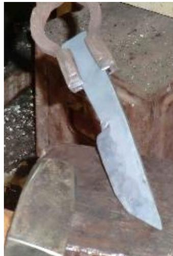
Eventually, the spine will be straight and will “thump” along its length when the edge is struck. As you can see in this image, the spine is ok again and the heat distribution between spine and edge is obvious. As you continue to forge the bevels, continue to straighten the blade as needed. Guess what technique is absolutely critical when forging a single-edged sword like a katana....
