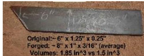
You can saw out the blank anyway you want but a horizontal metal cutting band saw and a pair of Vise-Grips makes this a snap. Since a nice look at the end of the tang is also a slant, you can saw out trapezoids and minimize stock waste as well as save some time at the anvil.
