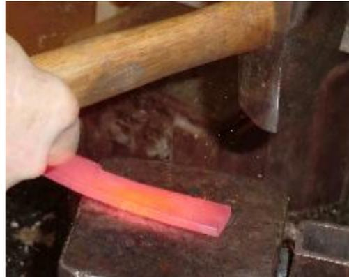
this. Flip the blank around and start heating the blade section.
