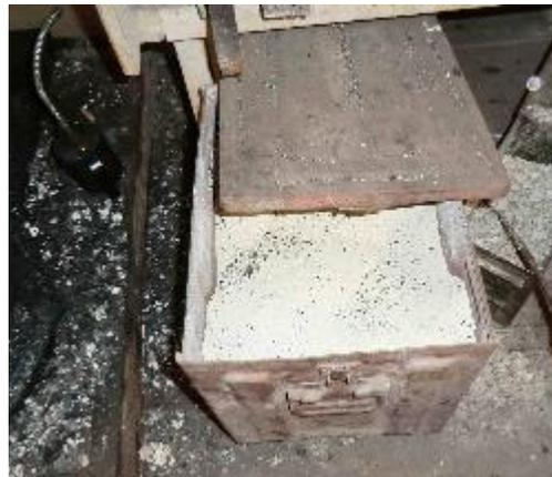
Vermiculite (here in a cannon shell casing – got to love military surplus!). In either case, let it rest for at least an hour or more (until cool to the touch). You can also use an electrical digitally programmable oven (like a Paragon) and run a typical 13 hour program. For most of us, the ash or vermiculite is sufficient. On occasion, when dealing with O1, the industrial process may be required.
