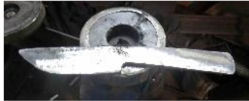
The next stage is to profile the blade. I typically follow the sequence shown – first the spine over the blade, then the spine over the tang (blending them as needed), then the edge, and finally the bottom and end of the tang. You are going for a surface at more or less right angles to the sides of the blade and tang.
