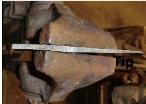
What we now have is a rough blade (note – there is still a small amount of curve present), and it's time to work on the tang. The tang can be forged with a top-to-bottom taper (simplifies some grinding and improves balance while complicating fit-&-finish) or left quasi-rectangular in cross-section. It should taper from the blade to the tip.
