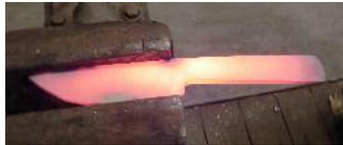
A couple of taps on the back corner of the tang drops the tang a touch and makes the blade feel better in the hand (IMHO).
