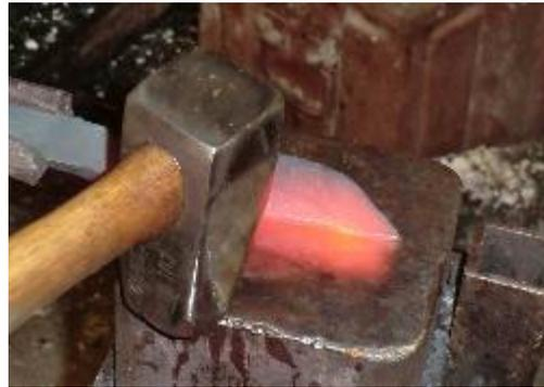
There is nothing special about the spine. You can place the edge in contact with the anvil and hit the spine to clean up hammer marks and level the spine. You can also work the tip as shown to correct the hook or to create a drop point or clip.
