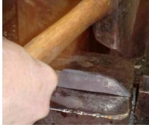
Here you can see that there is some deformation on the edge but the spine is getting close to being where it should be.
