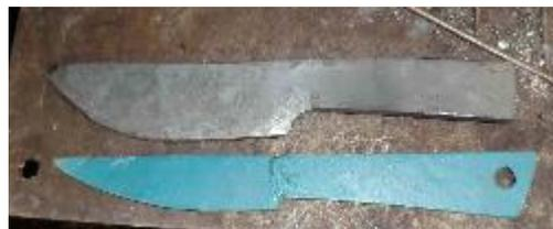
After forging, it is longer. Note that while we started with 6" of stock, the rough forged knife is now approximately 9.5" long. This is one of the reasons I like to forge blades. Once the tang is done, so back and make a final pass on the blade. Clean up hammer marks (switching to a lighter hammer helps here), correct any problems of the bevels not being centered, and check and correct the taper of the spine relative to the center line.
