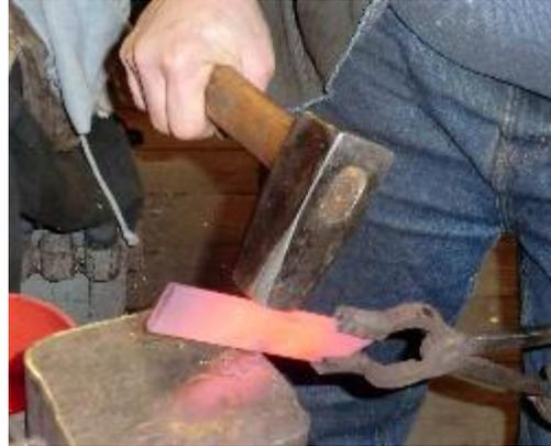
In this case, the depression is barely a suggestion. This technique works but has two drawbacks – the actual angle of the depression to the blade is not optimal and the spine of the blade will have been pushed down towards the depression – something that will have to be corrected later. There is a better solution if you happen to have available...
