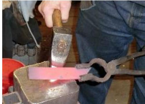
A treadle hammer, a striker, or a fuller. As shown, a piece of round stock is simply beaten into the blade at the delineation point. It doesn't (and actually shouldn't) have to be more than 0.5" deep.
