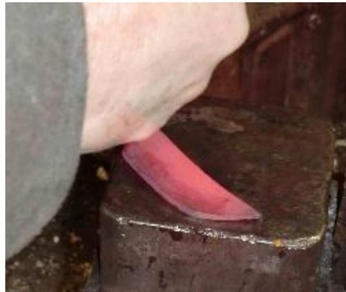
Flip the blade edge up and across the flat of the anvil. Hammer straight down onto the edge. Yes, it will deform but the spine will begin to straighten. If the blade is too cool to move much, just stop working on the edge a bit sooner and then follow this procedure. You want to keep an eye on the degree of “hook” and correct it when it looks like there is maybe a quarter inch or so of air.
