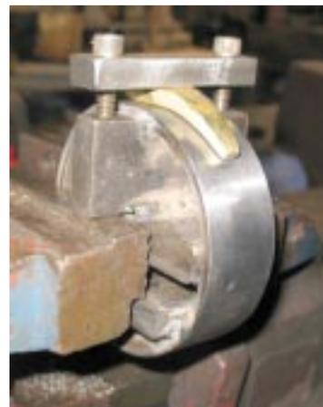
used machinist's clamps, hard wood wedges driven into the slot and an altered cheap drill press vise (below, left). I replaced the thin vise jaws from a 2.5" Harbor Freight vise with blocks of mild steel. The blocks were drilled and threaded to accept 8x32 cap screws. The guard can be laid down between the cap screws and the vise closed to hold the guard securely. It's then off to the surface grinder, belt grinder and/or buffing wheel to get the guard into the final polish.
