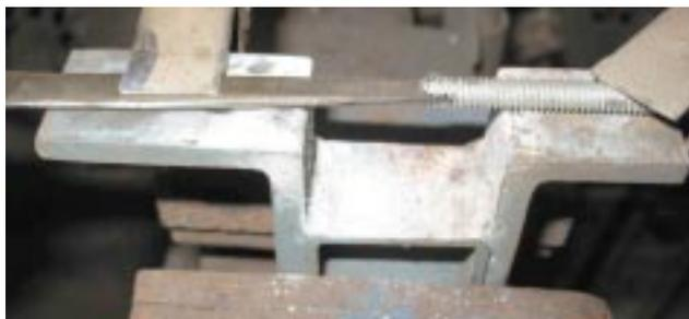
It's basically a couple pieces of angle iron welded to a bit of rectangular tubing. The tang is clamped to one side and the bolt to the other. They join in mid air (the bolt is slotted to fit over the tang). A bit of borax and brass with the help of an oxy-propane torch fuses them together. While the heat is way less than welding, it still screws up the grain structure in the tang tip -- SO NORMALIZE!.
