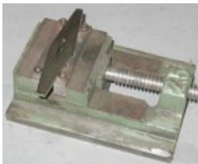
Drive it back onto the tang to get the final fit. By now, the slot is probably not perfectly in the middle of the block, so scribe the guard shape onto the block using the blade as a centering guide. Saw out the guard. The wrinkles now need to be removed, so there needs to be some way to hold the guard when grinding and polishing. I've
