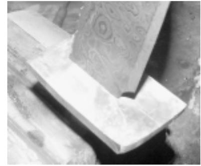
**Fig.8: Guard ready for soldering**
