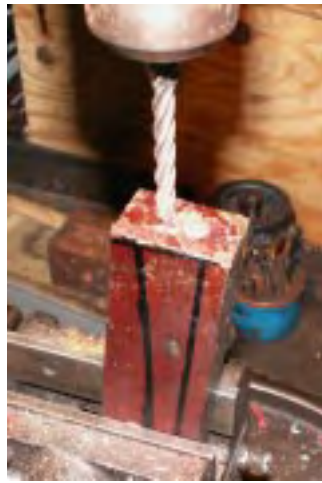
Fig.17: Drill flanking holes
