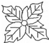
Cut the 4 rosettes from 16-gauge sheet steel and use a chisel to incise veination patterns. Drill a 1/2" hole in the center and make short angled cuts in each leaf edge. Bend back the metal at the cut, creating a serration and a triangle of metal which can be driven into the wood to secure the rosette.
