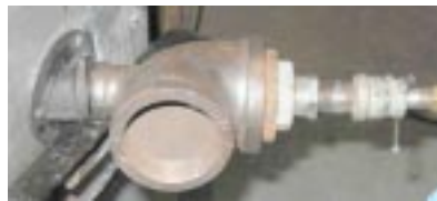
Figure 3: A Sidearm burner
