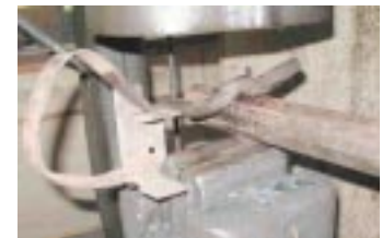
Figure 6: Swage in action
