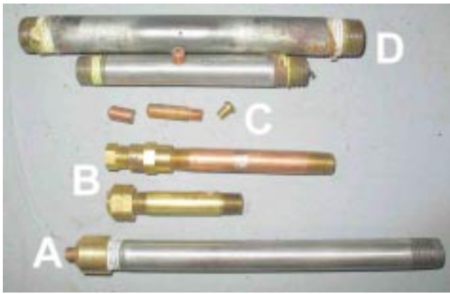
Figure 9: Gas delivery tubes
