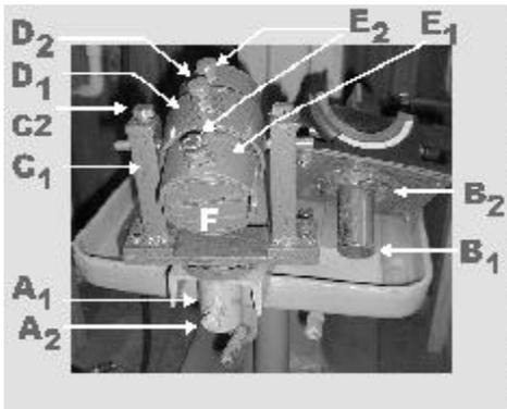
The combination of the socket, insert and plate gives a 360 degree rotation parallel to the ground. By making multiple plates and inserts, a variety of vises can be used in the same mount. On the knife-makers plate, there are two uprights ( $C_1$ ) with lock screws ( $C_2$ ). The uprights were made of square steel tubing with a plate welded on the top. The plates had a 1/2" x 13 nut welded on the inner surface.
