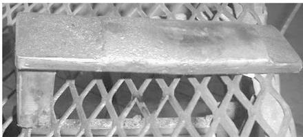
**Figure 9: Fullering plate**
