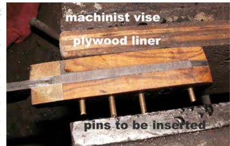
Fig. 8: Pin insertion
