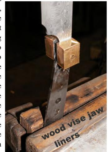
Fig.4: Soldering the bolsters
