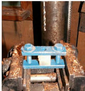
Fig.2: Bolster clamp on drill press
