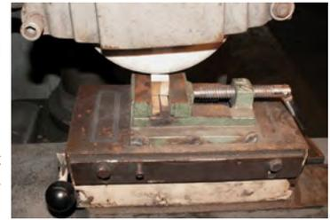
Fig.3: Grinding bolster surfaces
