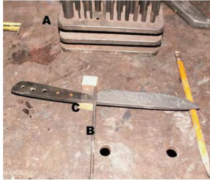
Fig.1: Marking the bolster rivet hole
