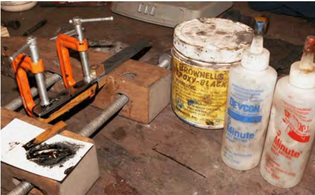
Fig. 6: Gluing the first side
