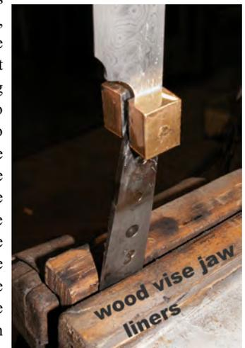
Fig.4: Soldering the bolsters
