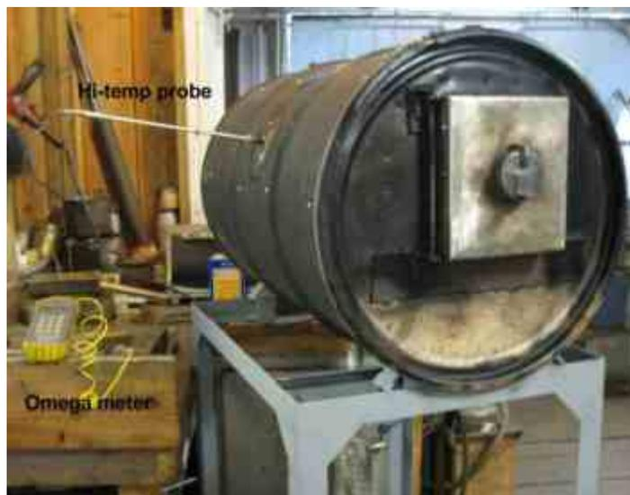
(showing temp meter & probe)
