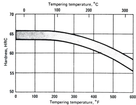
**O1: Hardness Versus Tempering Temperature.**
