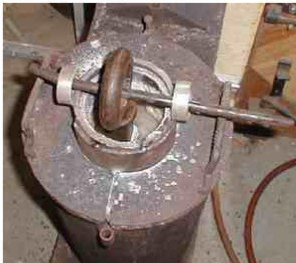
After several hours (long enough to generate banite), the low-temp salt is poured into a SS pan and allowed to cool. When cold, the block is broken up and place in the ammo can for next time. The blades are washed and stored awaiting the final grind and the hooks are washed and stored. The heat-treat shown here for thirteen blades took a total of five hours from start to finish.
