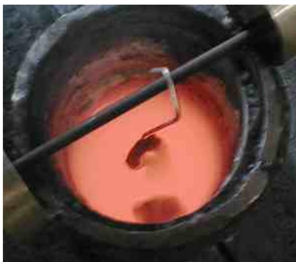
I wear welding leathers, an apron, gloves and a face shield anytime I'm near the pot (better sweaty than sorry!). I use tongs to hold the wire while sliding the blade into the lava pool. The high temp
