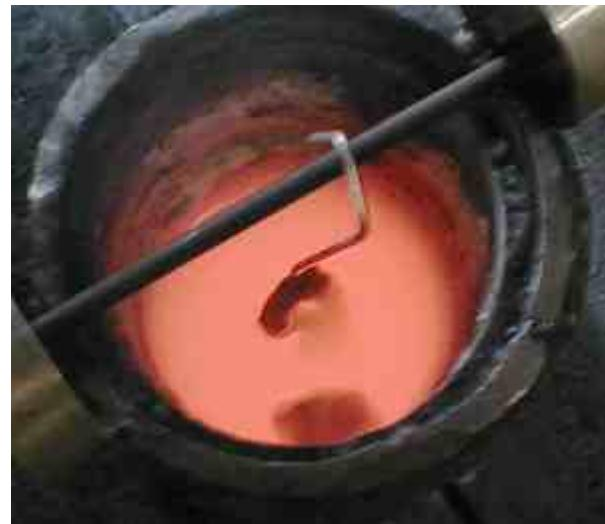
I wear welding leathers, an apron, gloves and a face shield anytime I'm near the pot (better sweaty than sorry!). I use tongs to hold the wire while sliding the blade into the lava pool. The high temp
