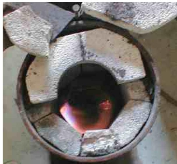
Once the low-temp pot is stable, the burner is lit off in the high temp forge using a piece of flaming newsprint and about 8 psi of LP. You can see the flame swirl in the shot to the right. Once the forge warms up, the tube is lowered into the forge (the donut of bricks is already in place) and the clamshells swung to the shut-and-support position.
