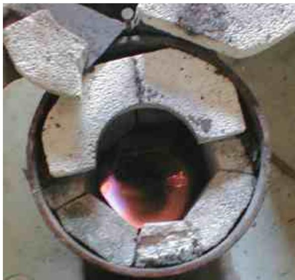
The temperature is monitored with an Omega digital temperature meter with an 18" long Type-K probe (~\$100 for the set). The picture to right shows the salt at 1367 F approximately 45 minutes
