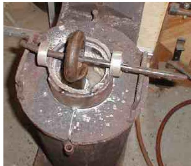
After several hours (long enough to generate banite), the low-temp salt is poured into a SS pan and allowed to cool. When cold, the block is broken up and place in the ammo can for next time. The blades are washed and stored awaiting the final grind and the hooks are washed and stored. The heat-treat shown here for thirteen blades took a total of five hours from start to finish.
