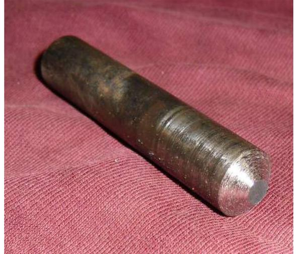
This is a close-up of the grinding jig and one of the blanks after the grind. Repeat for as many as you need (at least two).
