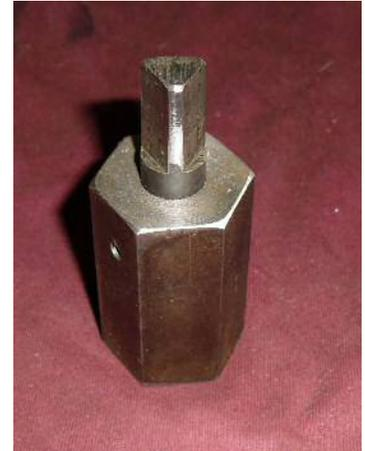
The next step is heat treating. I used oil hardening drill rod (O1), so all I did was use an oxy-propane torch to bring the blank up to critical temperature (1500° F by eye), then submerge it in quenching oil. The butt end was held in a set of tongs for this process. This is – to be generous – slapdash but sufficient for our purposes here. The blanks were tempered at 375° F for an hour, so the final hardness ought to be in the lower 60's (Rockwell C).
