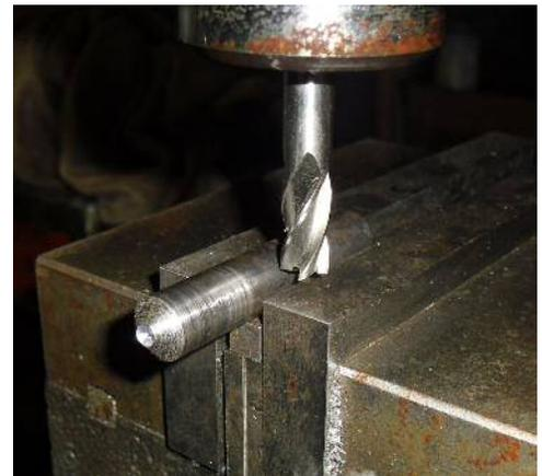
If you have ever used the drill bits that have a more-or-less triangular end, you know how well they work in a drill chuck. The same idea can be applied to the spinners. Get some scrap hex material (a big hex nut would do in a pinch), drill a 1/2" hole in the center, add a couple of set screws and you get the jig shown here.
