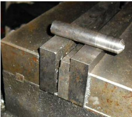
shallow pass with the end mill creates the first flat. By turning the blank over such that the tool bit is snuggled into that flat and making sure the bit is still flush to the side of the jaws, the blank is ready for the second flat. As long as you start the cut in the same horizontal position, the flats will be of equal length and opposite one another.
