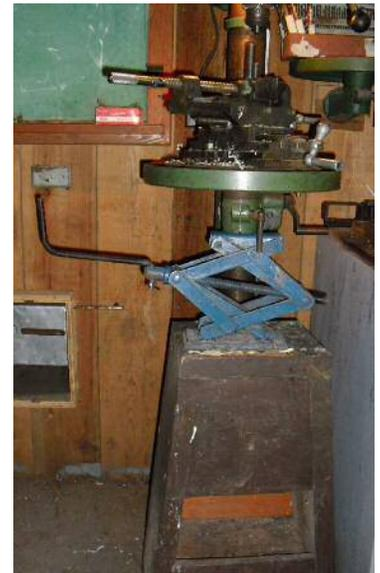
The upper and lower components need to be aligned. You can just eye-ball that or you can fish that piece of pipe used with the transfer punch mentioned above out of the scrap bin and use it as an alignment tool. Lock the lower unit in the cross slide vise and slip the pipe section over it. Adjust the X-Y directions of the vise until the upper spinner can slide into the pipe. Lock the vise and the system is aligned and ready for use.
