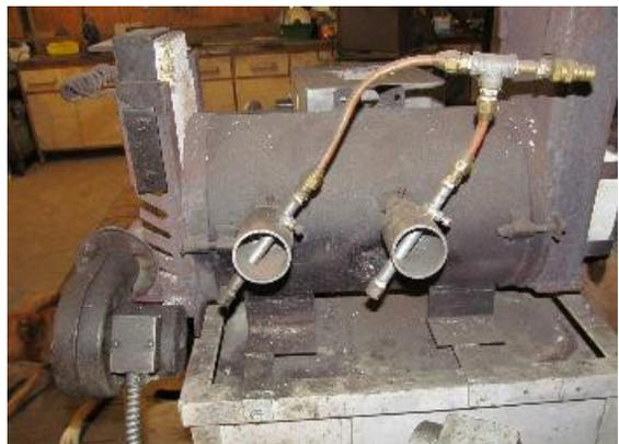
The blower is a 120V squirrel cage from the Surplus Center and is not particularly powerful. It talks to the manifold through a aluminum dryer hose. The switch on the leg controls both the main and the lateral blowers.
