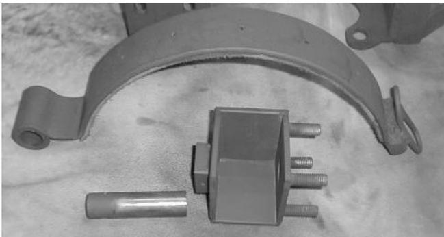
**Fig.2: Brake shoe & mounting box**
