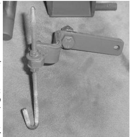
**Fig.6:Control arm (from front)**
