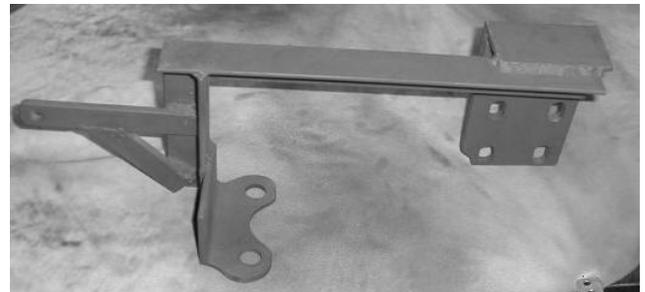
**Fig.5: Mounting arm (from behind & above)**
